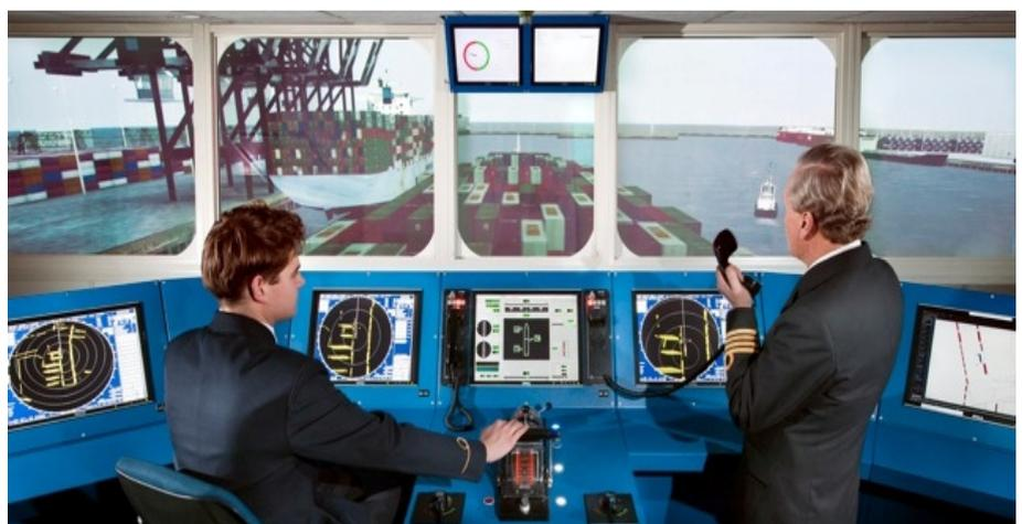
This is a fully equipped bridge with 360 degrees visual projected scenery. A mock-up of a real ship bridge is located in the centre of a cylindrical projection wall on which the graphics image is projected. The diameter is 20m and the bridge house is approximately 8m by 6m. The bridge is equipped with realistic consoles and instrumentation, including bridge wing consoles. Bridge and console layout can be adapted according to client wishes or research needs.
