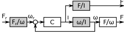
Fig. 3. scheme to calculate the thrust based on the requested thrust. Gray blocks are known. The lead-lag controller is designed to have a bandwidth of 10 Hz
