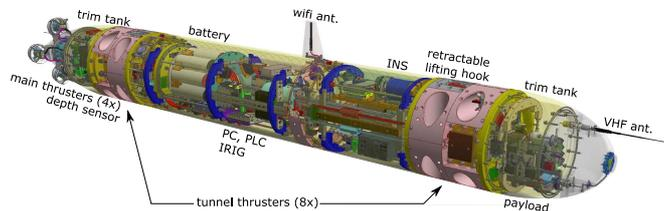
Fig. 1. A CAD drawing of the MAUV
