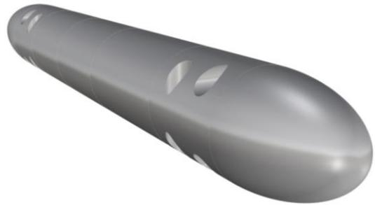
Fig. 2. Hull geometry of the mAUV (view from the bow)
