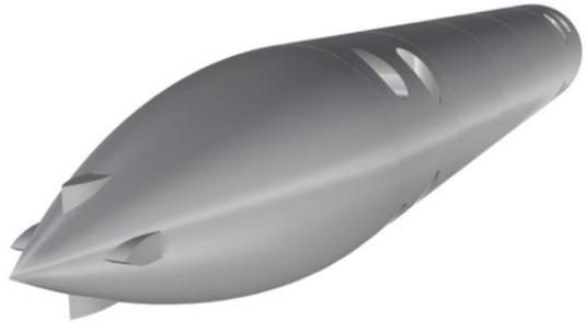
Fig. 3. Hull geometry of the mAUV (view from the stern)
