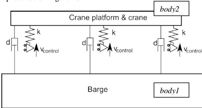
**Figure 16: schematic representation of Barge Master**
