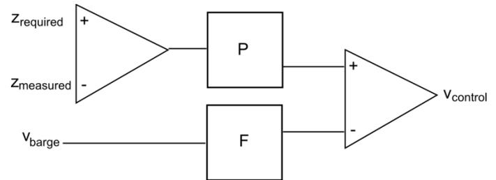
**Figure 9: simplified representation of the control system**
