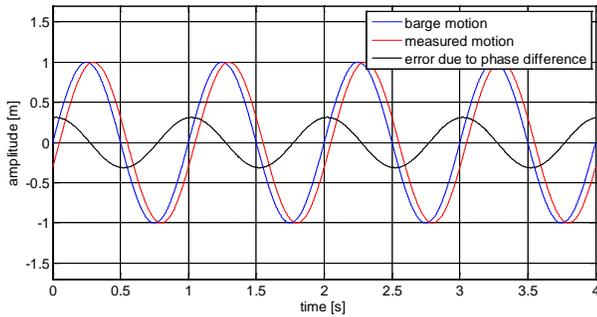
**Figure 10: residual motion for a 18 degree tracking error**
