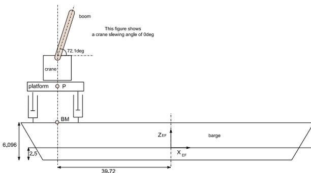
**Figure 5: General arrangement of the barge and barge-master platform**
