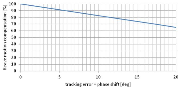
**Figure 12: theoretical compensation vs. tracking error**
