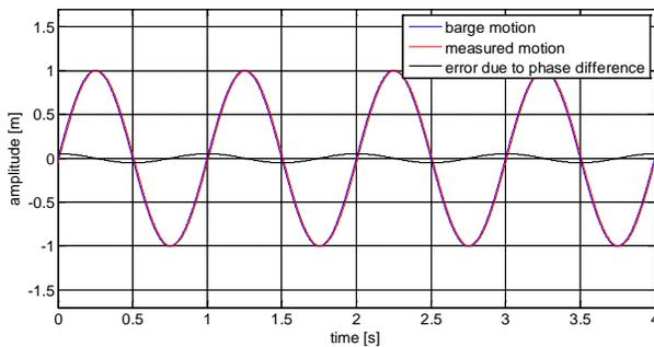
**Figure 11: residual motion for a 3 degree tracking error**
