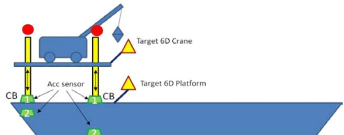
Figure 7: overview of the instrumentation
