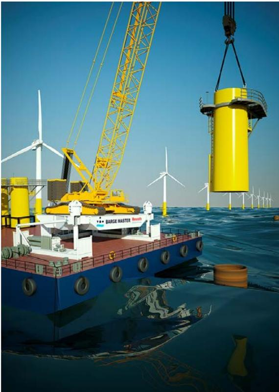
**Figure 1: application of the barge master for offshore installation operations**
