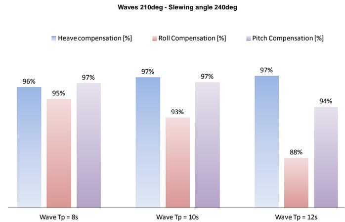
Figure 13: bar chart of the compensation performance measured with the optimized controller
