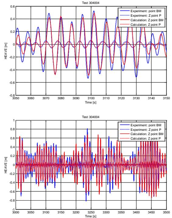
**Figure 17: comparison of the heave time trace : experimental v.s. numerical results**
