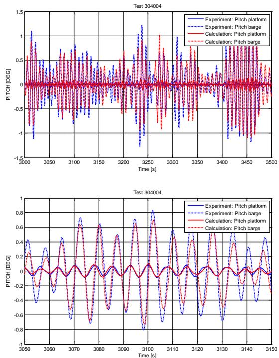
**Figure 18: comparison of the pitch time traces: experimental v.s. numerical results**
