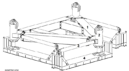
**Figure 4: isometric view of Barge Master with 1) platform 2) cylinders 3) constraints 4) foundations**
