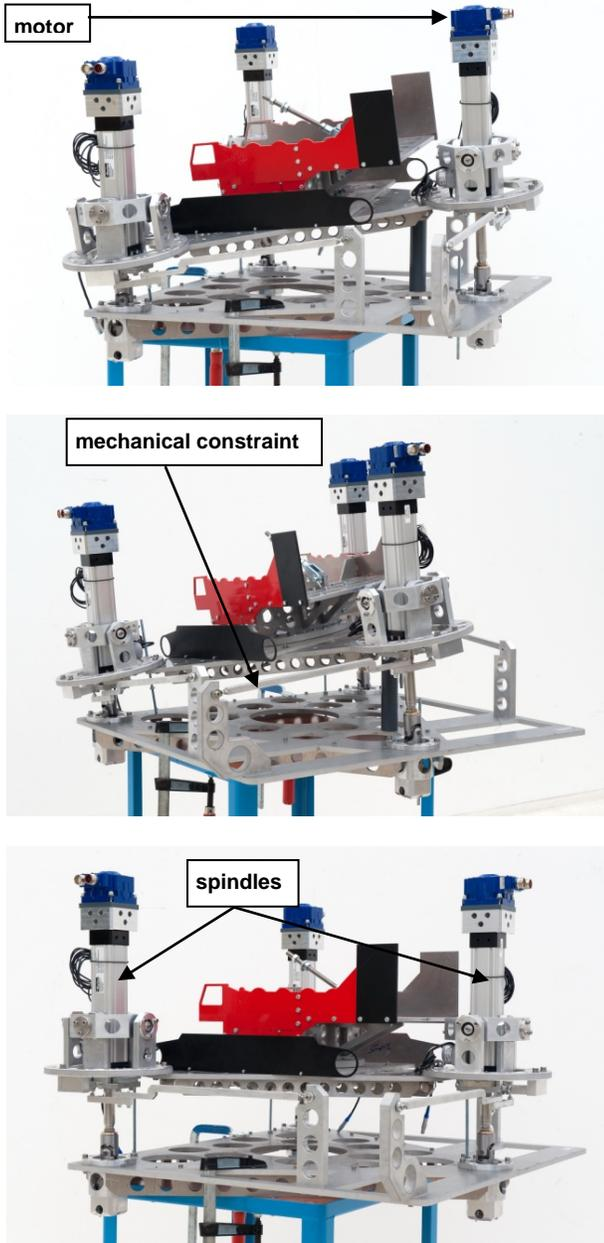
Figure 6: photographs of the Barge Master model
