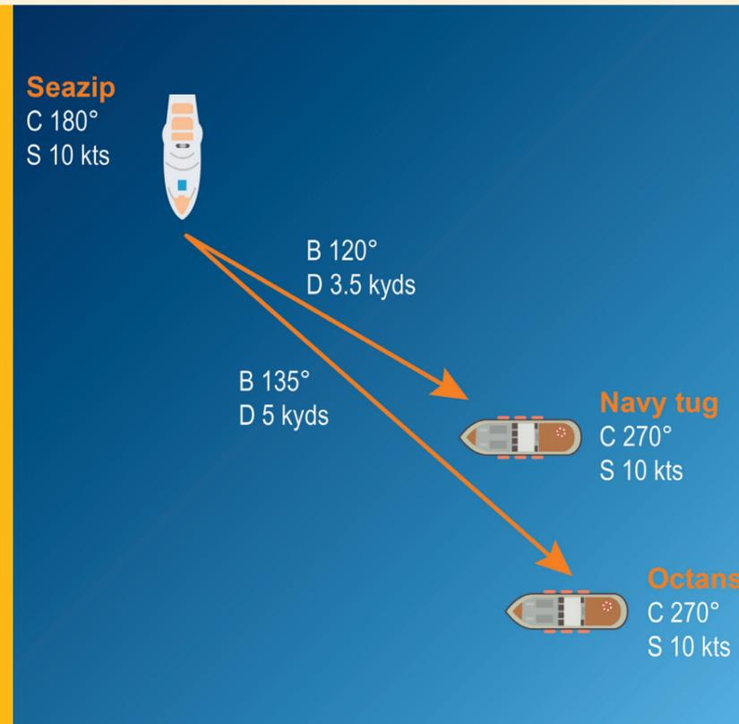
Figure 1 Typical 'open water' test scenario of more or less equally sized vessels
