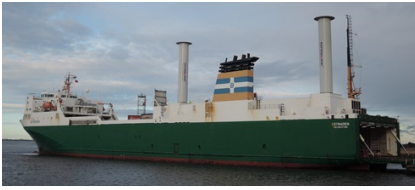
Figure 2: Example existing installation: Norsepower rotors on Bore's Estraden (picture by Norsepower)
