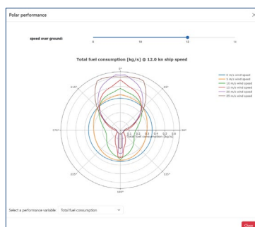
Ship performance polar (left) and average fuel consumption over a route with and without wind propulsion (right).
