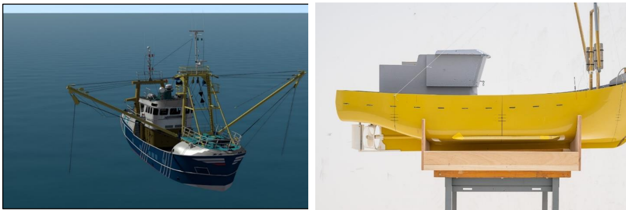
Figure 3-1: Visual of the fishing vessel in the simulator [left] and picture of the scale model [right]
