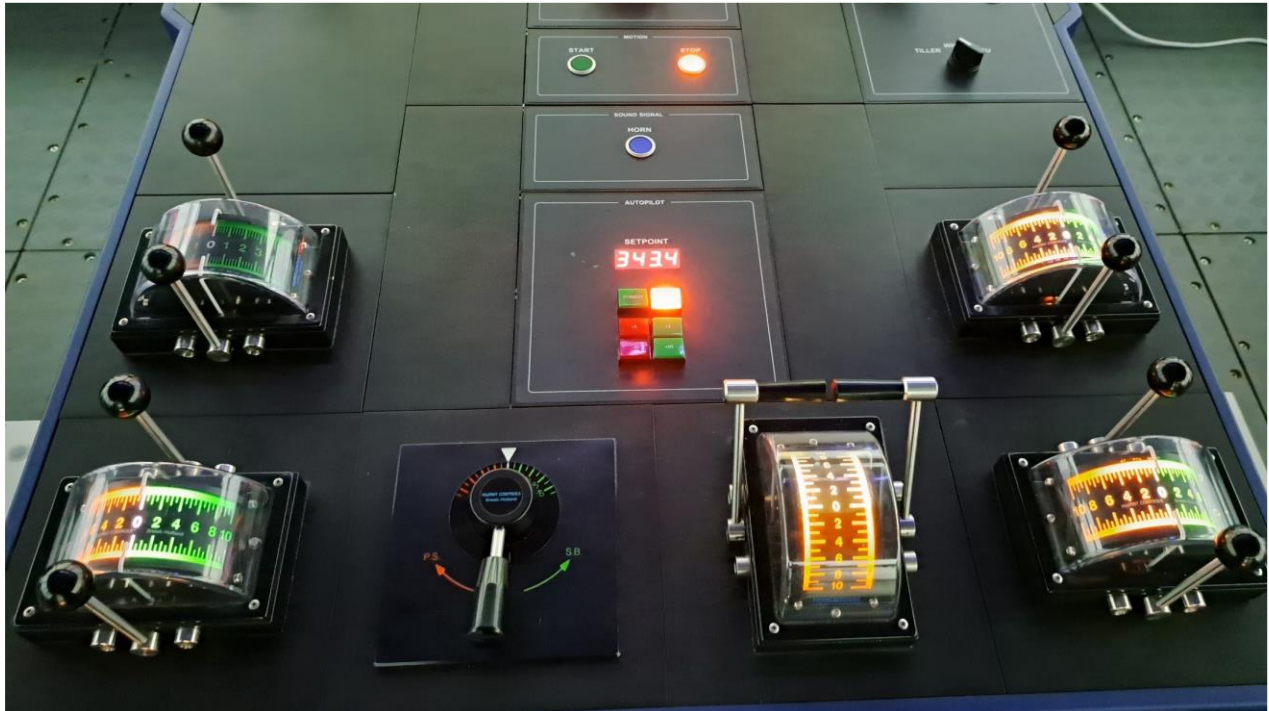
Figure 3-7: Control panel with autopilot, telegraph, rudder and winch controls
