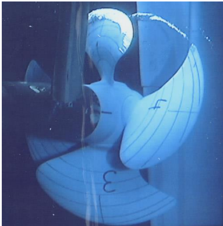
Figure 2-6 - Cavitation on a model propeller taken in MARINs testing facilities.
