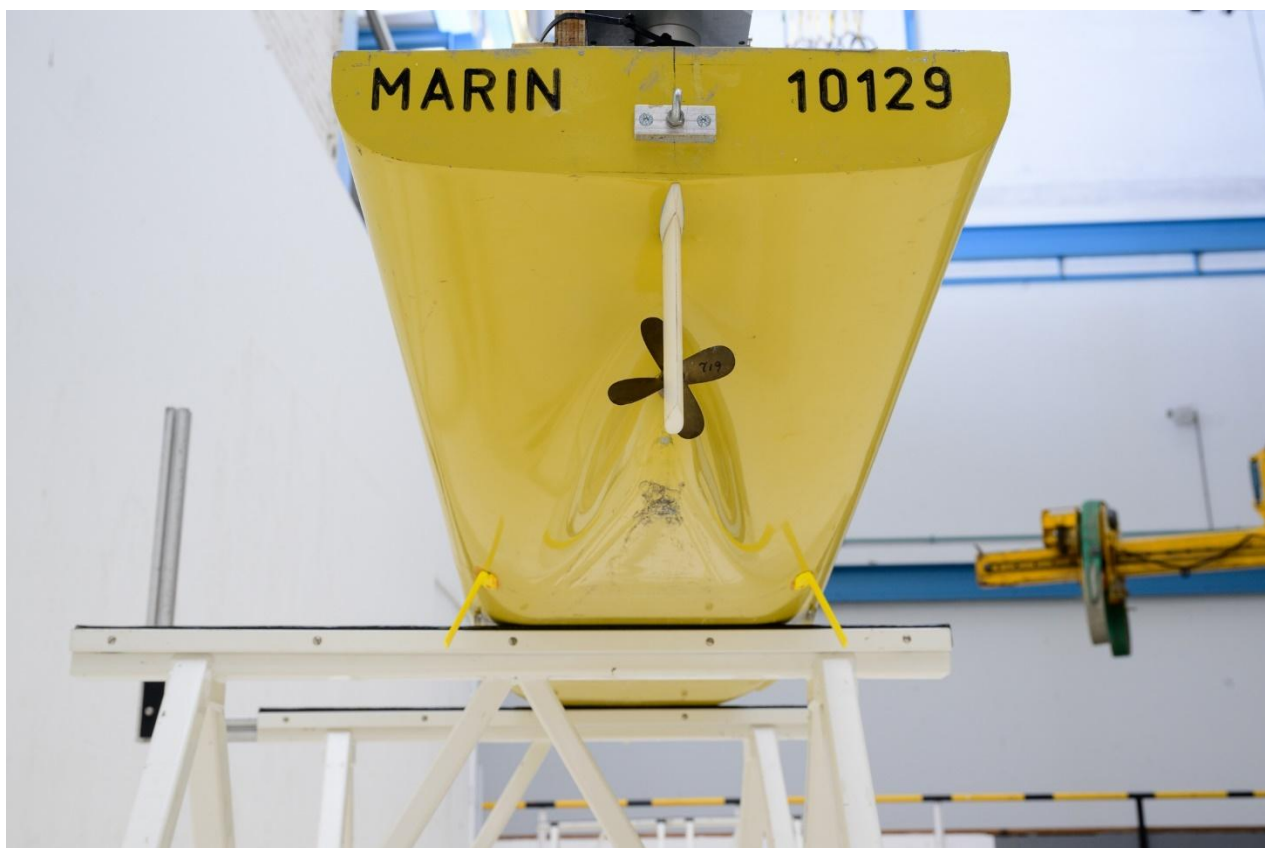
Photo PH8: Details of the rudders and propellers
