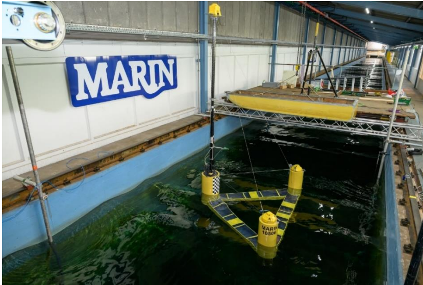
Figure 2-7: Overview photograph of the model in the MARIN concept Basin.
