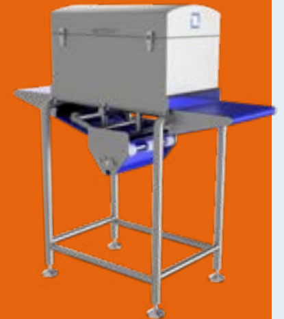
The conveyor belt used in fish processing with the “vision robot” that performs the measurements and collects data.
