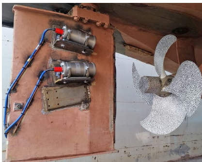
Stereo digital image correlation (Stereo-DIC)
