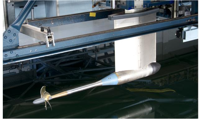
**Figure 4: The experimental open-water propeller test setup.**
