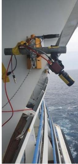
**FIGURE 3:** Side view of the port side camera. The other camera can be seen in the distance.
