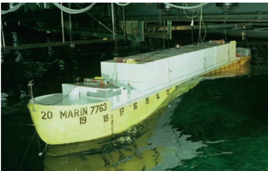
Irregular seas, wave direction 240 deg. H = 3.75 m. T = 8.35 s. Zero speed
