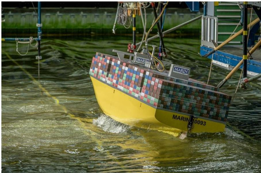
In the present task the seakeeping of ULCS's will be investigated to establish the extreme behaviour and the motion envelopes. Voyage simulations with GULLIVER will be used as a core tool to determine the motion envelopes. At this stage such simulations are foreseen for an NPX container vessel at a range of operational profiles (loading/stabilities) on two shipping routes (Far East - Europe and Trans-Pacific). The voyage simulation tool will be fine-tuned using model test results.
