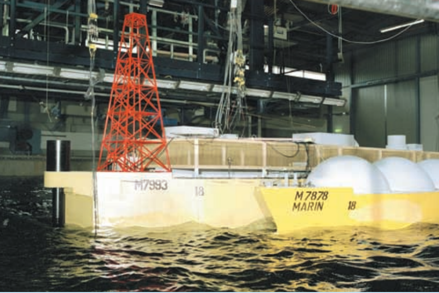
In the process of confirming the feasibility of side-by-side offloading operations of the Shell Floating LNG System at the Sunrise field, in 1999 Shell commissioned MARIN to perform numerical simulations and model tests.
