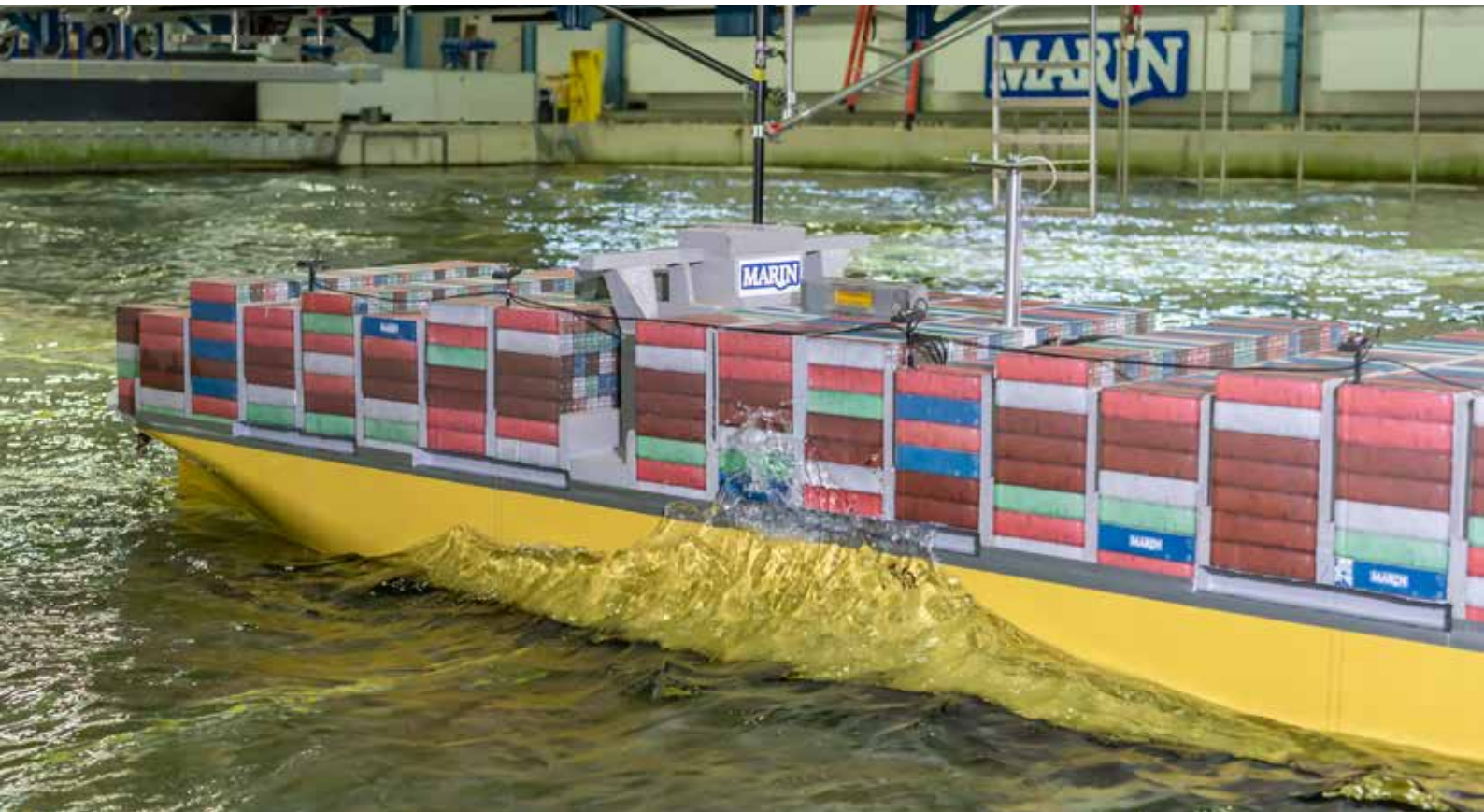
Scale model in 6.5 m high beam waves, water depth 21.3 m
