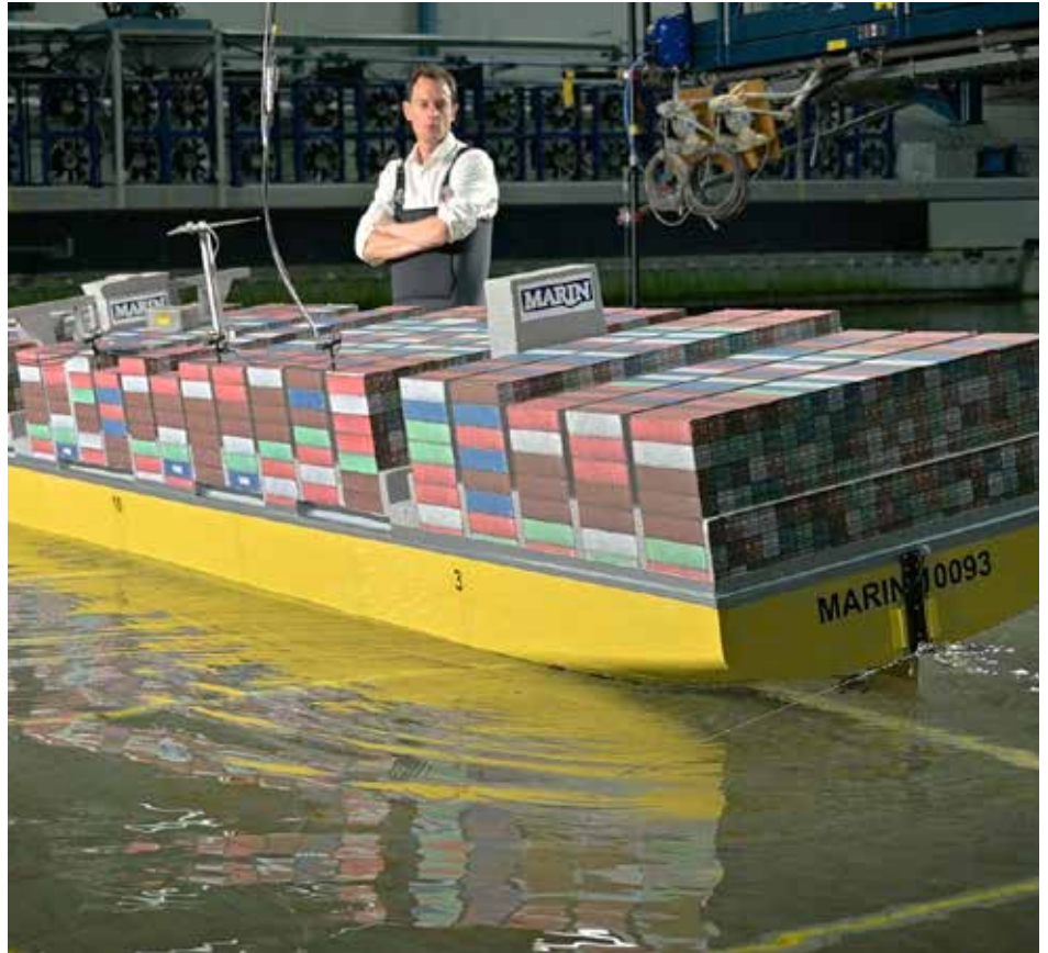
Scale model sailing at 10 kn through 6.5 m high beam waves, water depth 21.3 m
