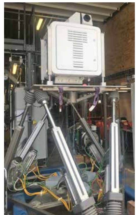
Lidar scanner on hexapod to simulate ship motions
