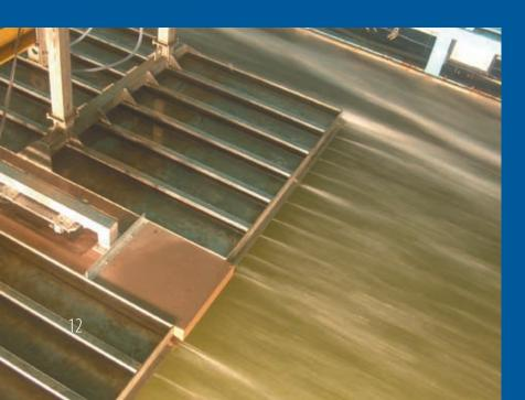
For PELS' free sailing model experiments in calm water, MARIN's Depressurised Towing Tank was used. In this way, the compressibility of air was found to be responsible for several measurable scale effects on the micro and macro scale of air- lubrication techniques.
