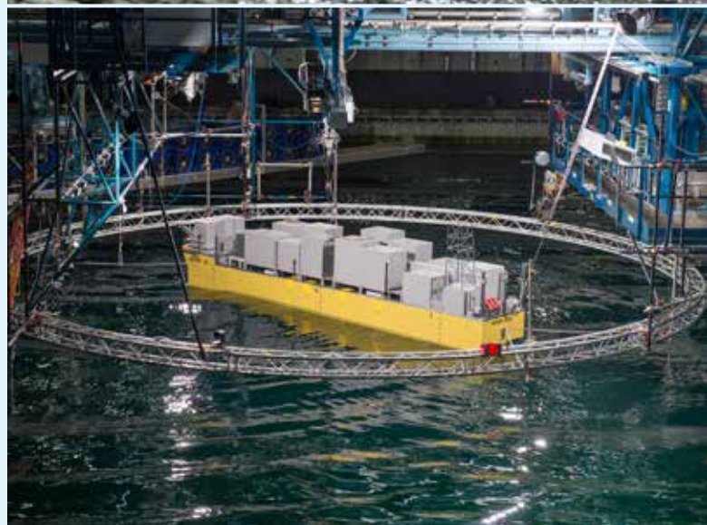
Seakeeping model test in bow quartering wave
