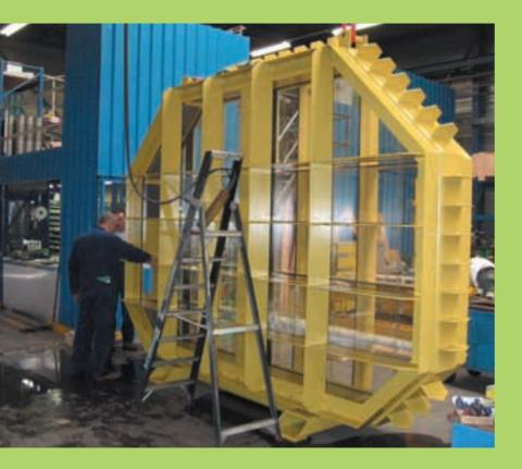
study complex free surface problems, which is flexible in its application and has a coupling possibility to the other tools of participants'. As part of the validation, this year 2D sloshing experiments are to be carried out at large scale I:I0, resulting in a tank of 3.9 m wide and 2.7 m high. These will be used for validation of the 2phase flow models in ComFLOW. Contact: Tim Bunnik (t.bunnik@marin.nl).
