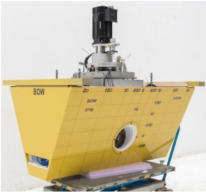
Test set up for mechanical drive tunnel thruster
