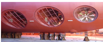
Combination of mechanical and RIM driven tunnel thrusters. Photo: courtesy Brunvoll AS
