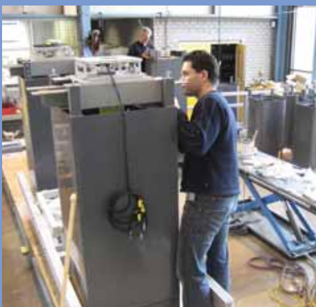
MARIN engineers prepare the building block model of the semi-submersible
