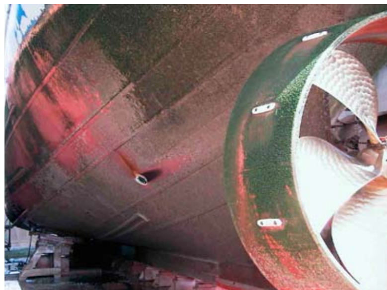
Severe fouling by green algae and barnacles on ship hull and propeller tunnel
