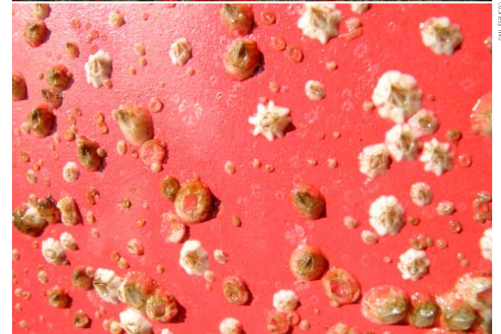
Adult barnacles of various age at a raft exposure panel at TNO
