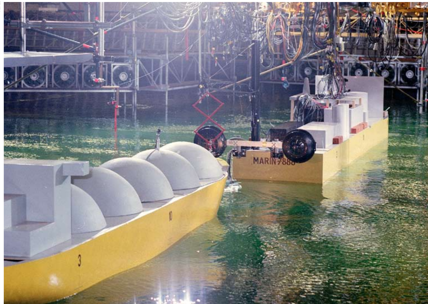
Tandem offloading test results from MARIN's offshore basin are used for verification of numerical models
