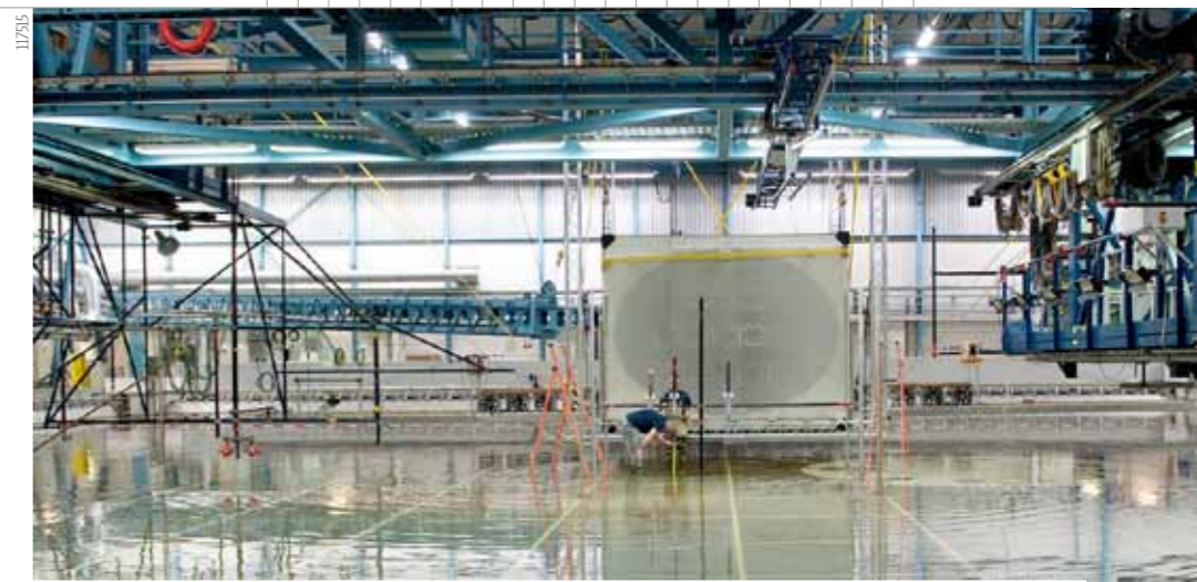
New wind set-up to test floating offshore wind turbines in Offshore Basin
