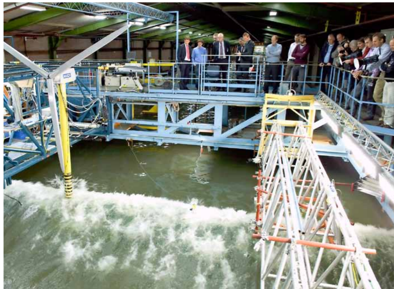
Breaking wave on a wind turbine scale model with realistic flexibility in the MARIN facilities during the Offshore Wind Seminar
