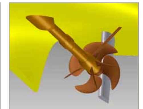
Illustration of a Pre-swirl stator for a twin-screw vessel.
