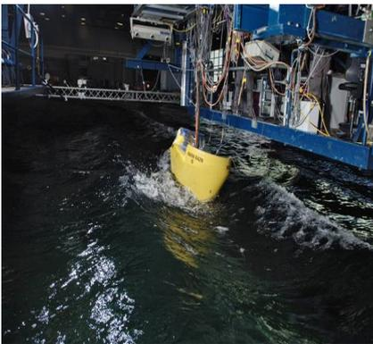
Model test of an offshore support vessel rolling in beam waves
