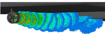
Wakefield development behind an azimuth thruster (PIV measurement)
