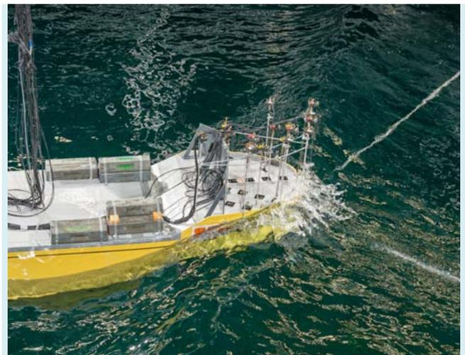
A typical example of concept modeltest was the test series performed for SBM. A green water assessment was made in the Offshore Basin. For these tests a tanker from MARIN's stock was used with a large number of wave probes at the bow. Adjustments to the test conditions were realized directly responding to the test results.
