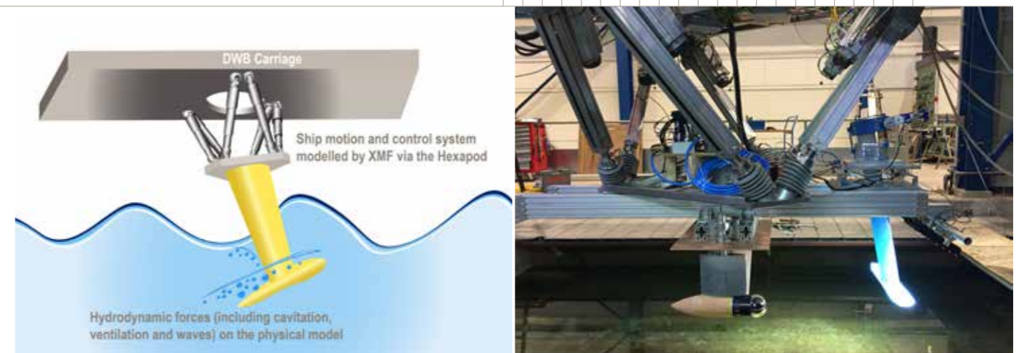
Figure 2: Model test set-up with hexapod and hydrofoil (left) and set-up as tested in Depressurised Wave Basin (right)
