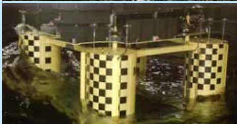
Wave impact at wave ward column
