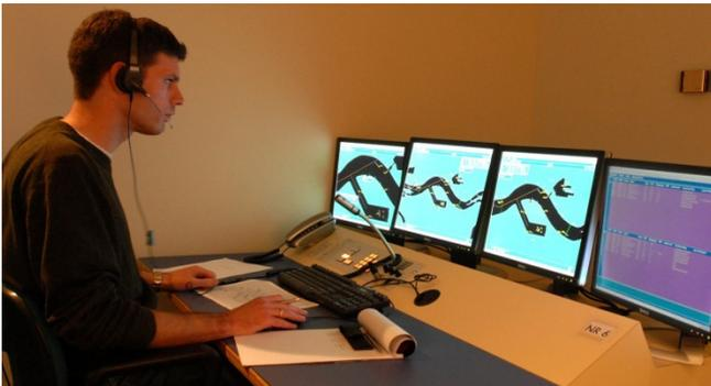
By combining all six cubicles of the VTS operators, a traffic control centre or even a network of control centres can be simulated. The training scenario has been computerised in such a way that the instructor can interfere manually with the exercise at any time. Ships can be in an automatic or manual control mode. In the latter case the instructors control the ships and play a major role in the communication between VTS operator and all ships that are present in the trainee's (block) area.
