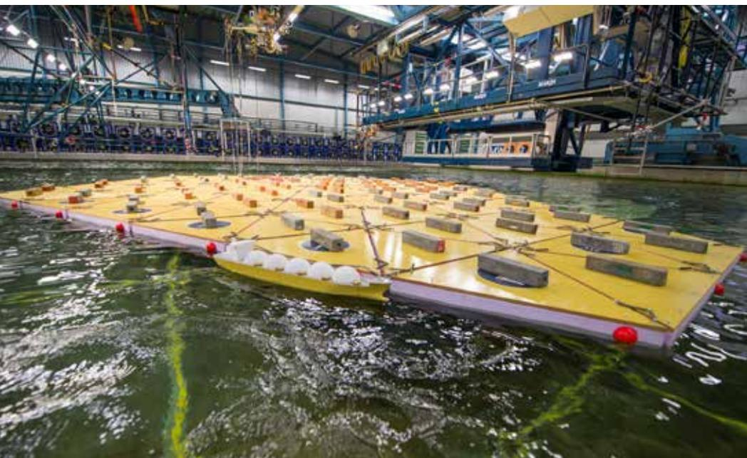
Due to rising sea levels and the increasing global population in coastal areas we need to use our oceans more for food production, working and living. MARIN has recently tested an innovative concept for a floating mega island, which comprises 87 large, floating triangles that are connected to one another. Together they form a flexible island that can be as large as 1-5 km in cross-section.
