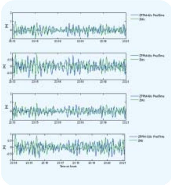
Vessel heave motion measured versus predicted 42, 60, 90 and 120 sec. ahead
