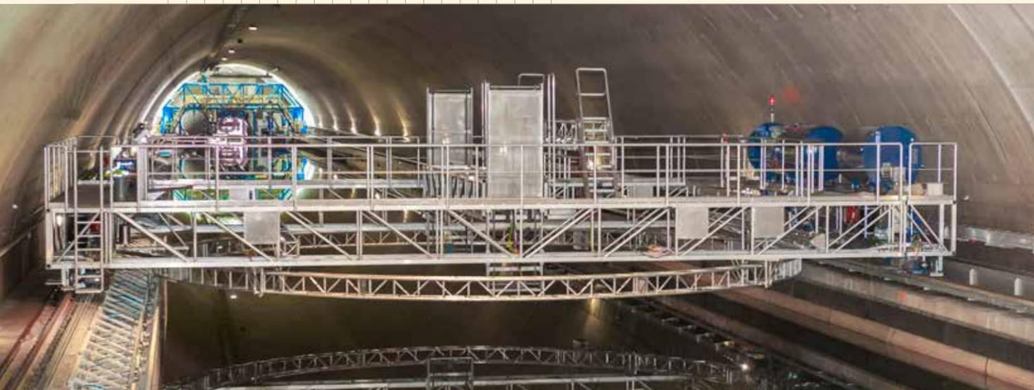
Silent towing carriage in the Depressurised Wave Basin
