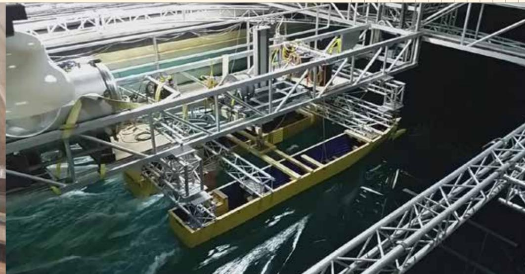
Silent towing carriage towing a model
