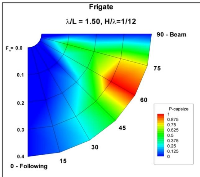
Capsize probability of a frigate as function of the wave direction and Froude number
