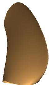
INDFACT incorporates an iteration procedure which combines cavitation on both sides with a strength calculation. It produces chord length, section thickness and camber distributions.
