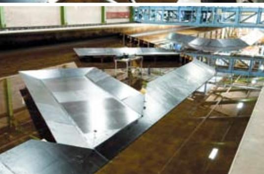
Harbours being built-up (top-down): construction of main waterways, secondary shipping channel, two barge docks, final test set-up
