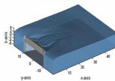
**Modelling of the Green water concept with diffraction theory and ComFLOW simulations**
