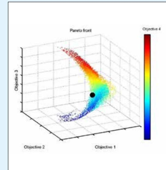
4D Pareto front of optimum propeller designs with arbitrary objectives
