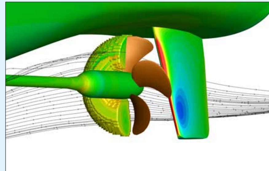
RANS-BEM coupling with propeller modelled by body forces
