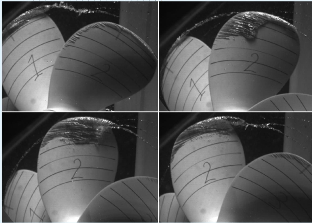
High-speed video footage of propeller cavitation
