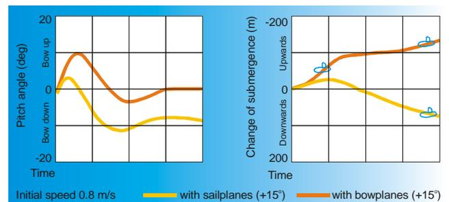
Diving manoeuvre at high speed due to 15 deg. rotation of forward planes for two hull configurations
