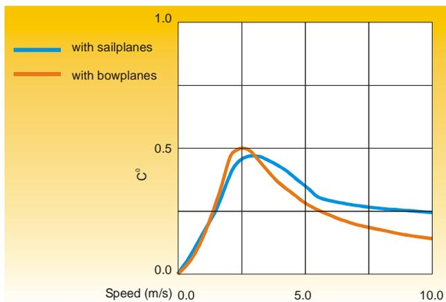
Dimensionless critical damping  $C$  of the vertical behaviour of two hull configurations
