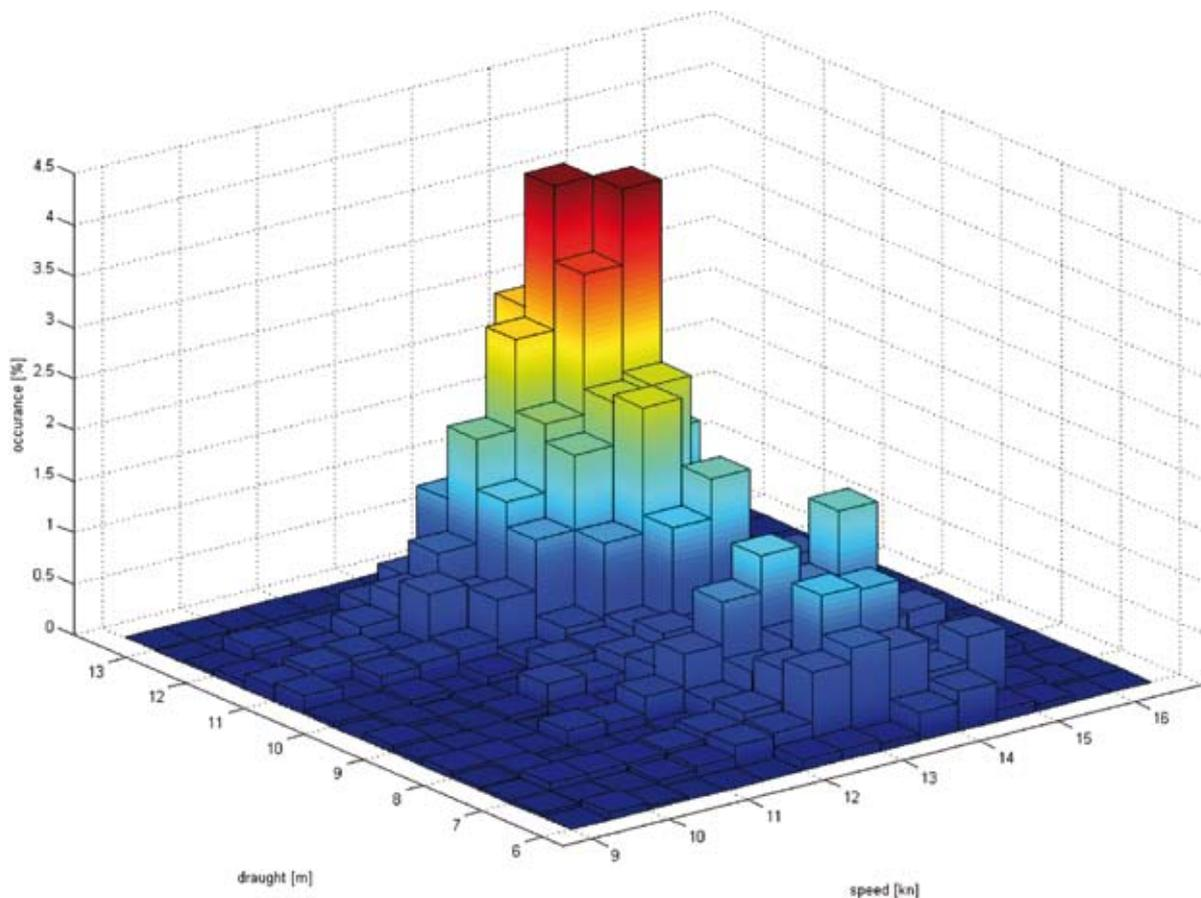
Figure 1: Operational profile of a tanker
