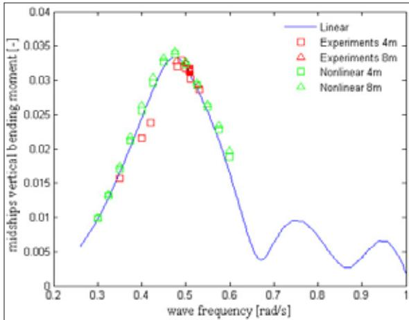
Figure 6. RAOs obtained from calculations and experiments.
