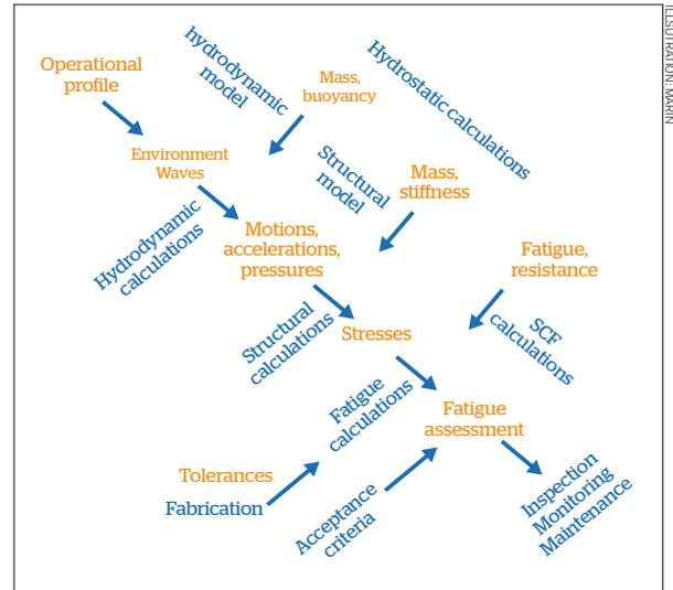
Figure 1. Elements of fatigue design
