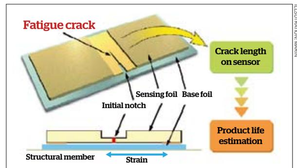
Figure 2. Illustration of the Fatigue Damage Sensor (Courtesy Kawasaki)
