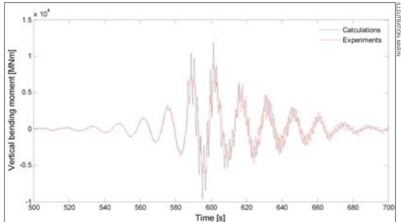
Figure 9. Comparison between the midships vertical bending moments due to whipping, as obtained from calculations and experiments.
