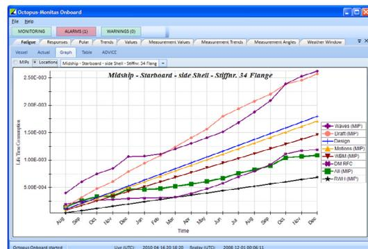
For the FPSO Glas Dour the Life Time Consumption is checked depending on the following parameters:
