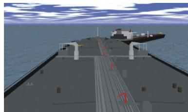
Manoeuvring simulation of crude oil tandem offloading
