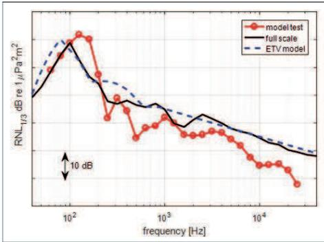
Figure 2: Comparison between model test, full-scale measurement and computation of URN of a merchant vessel
