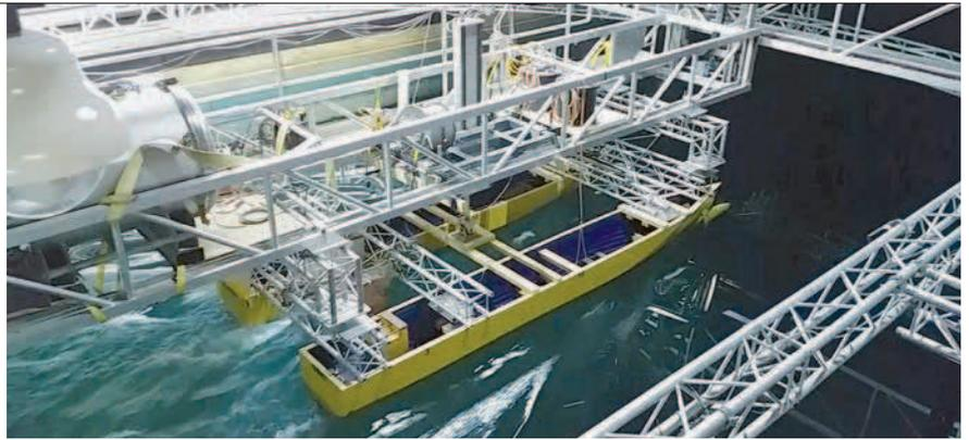
Figure 3: Silent towing carriage towing a model
