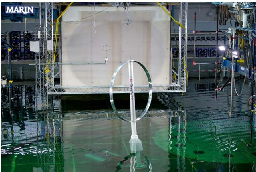
*The Deepwind floating wind turbine scale model in front of MARIN's dedicated wind setup*
