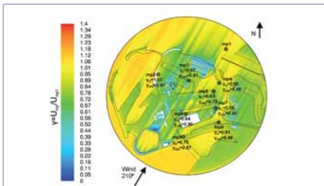
Figure 3: Result of CFD simulations for Port of Rotterdam: contours of normalised mean wind speed in horizontal plane at 15 metres above mean sea level (normalisation is performed using the wind speed at mp1)
