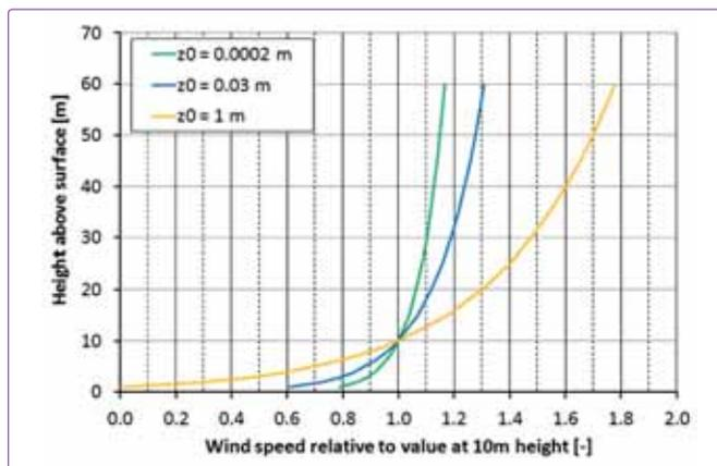
Figure 4: Logarithmic vertical wind profile for different surface roughness.
